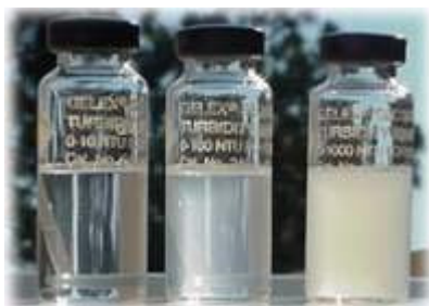
Figure 5.1 Turbidity standards of 5, 50, and 500 NTU
